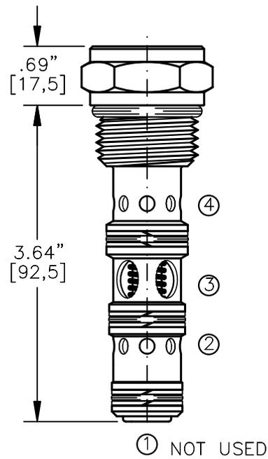
PORT #3 (INLET) IS ONE SIZE LARGER THAN PORTS #2 & #4 (OUTLETS).
