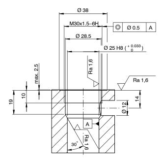
Cavity is manufactured with conventional tools (no form-tools available).
