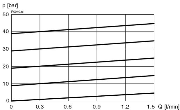
$p = f(Q)$  Druck-Volumenstrom-Kennlinie  $p_N = 100$  bar
