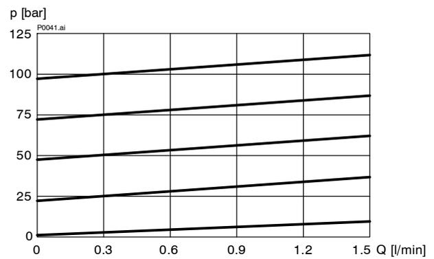
$p = f(Q)$  Druck-Volumenstrom-Kennlinie  $p_N = 160$  bar
