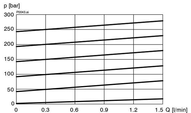
$p = f(Q)$  Druck-Volumenstrom-Kennlinie  $p_N = 350$  bar
