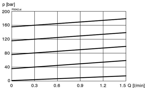
$p = f(Q)$  Druck-Volumenstrom-Kennlinie  $p_N = 250$  bar
