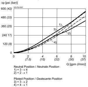
$\Delta p = f(Q)$  Pressure drop-flow rate characteristic
