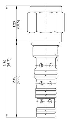
Version "S": adjustment screw (standard) <sup>3</sup> 5/16 (8) 3/4 (20)  $M_A$  = handfest angezogen (max. 49.1) max. 1.93 hand tightened 1 1/16 (27)  $M_{A} = 1$ ) () Ø0.755×0.097 (max. 112.3) max. 4.42 7/8-14 UNF-2A -€ ) Ø0.643×0.053×0.048 2.49 () Ø0.614×0.070 63. Ø0.643×0.053×0.048 3 A-1 ) Ø0.580×0.053×0.048 () Ø0.551×0.070 Ø0.580×0.053×0.048 0 Ø0.518×0.053×0.048 () Ø0.489×0.070 ) Ø0.518×0.053×0.048 1
