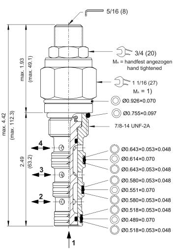
Version "S": Einstellschraube (Standard) Version "S": adjustment screw (standard)
