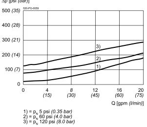
$\Delta p = f(Q)$  Pressure drop-flow rate characteristic  $\Delta p [psi (bar)]$
