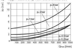
Δp = f (Q) Pressure drop-flow rate characteristic
