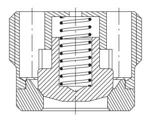
The new check valve is distinguished by it's guided valve poppet with internal spring. The stroke was increased to optimise the valve's Delta P values. The body and seat are press-fitted together and, like the poppet, are hardened.
