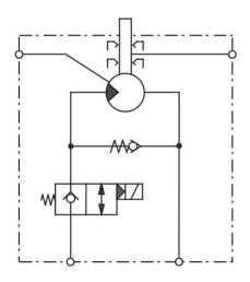
QXM internal gear motors with make-up valve, ON/OFF valve, external drain port, sealing variant for ultra-high protection against external leakage, and tell-tale hole.
