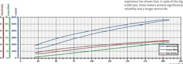
While continuous high speeds of more than 3,000 rpm are problematic for other motors, the QXM is just getting into its stride. Field experience has shown that, in spite of the high working speed of 6,000 rpm, these motors achieve significantly higher levels of reliability and a longer service life.
