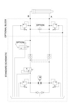
Thanks to its design, this mini power unit is also ideally suited for direct combinations of power unit + cylinder. As a result, the installation dimensions in machines can be significantly reduced, as there are no hydraulic pipes or hoses. It is also important to note that the UP40 power unit can be in-stalled either horizontally or vertically.
