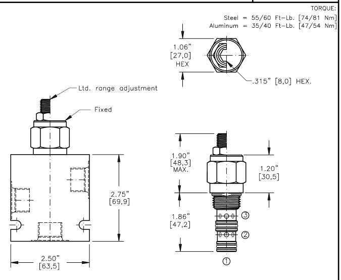
FOR ALUMINUM OR STEEL VALVE HOUSING CONFIGURATIONS SEE PAGE 0-032.1
