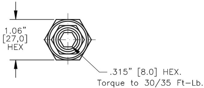
Turn screw clockwise to increase the pressure setting.
