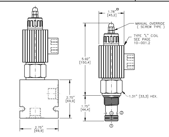
NOTES: SOLENOIDS AVAILABLE WITH DIODES — CONSULT FACTORY. TORQUE Steel = 75/80 Ft-Lb. [102/109 Nm] Aluminum = 55/60 Ft-Lb. [74/81 Nm]
