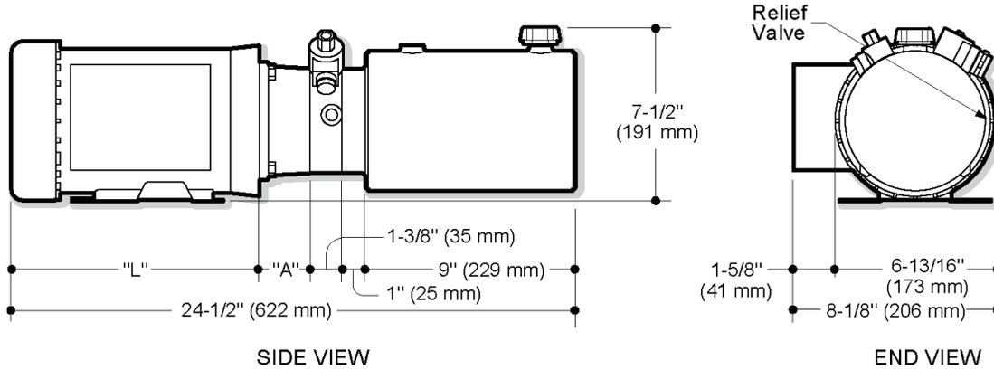
"L" dimension shown for 08751 motor is 10-11/16" (271 mm)
