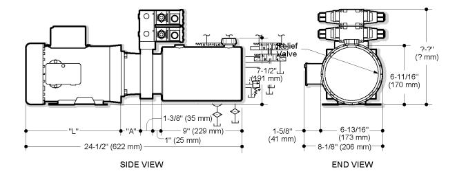
"L" dimension shown for 08751 motor is 10-11/16" (271 mm) "A" dimension for standard 01605 adapter is 2-5/32" (55 mm) "A" dimension for optional 01615 adapter is 3-11/32" (85 mm) Dimensions will vary according to motor output and manufacturer
