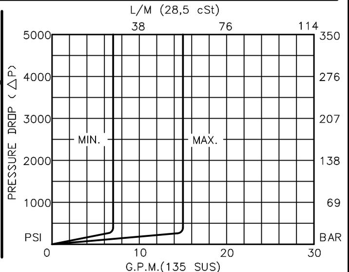
**FLOW CONTROL VALVE PRESSURE COMPENSATED,
