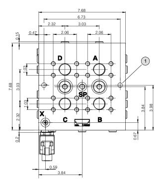
1 Clearance holes for M8 mounting cap screws to DIN 912
