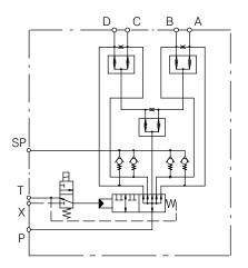
7.1.1.2 MT..DVV.....-EH-0T../02 With anti-shock valves (pressure-relief+make-up valves)
