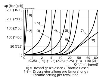
p = f (Q) Pressure-flow rate Adjustment, fine opening Measured via check valve
