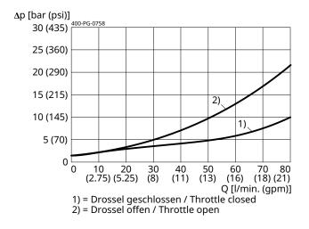
$Q = f(I:\Delta p)$  Flow rate adjustment
