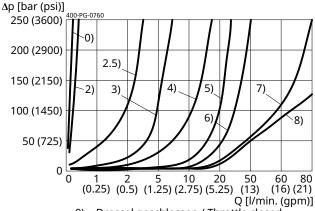
0) = Drossel geschlossen / Throttle closed 1-8) = Drosseleinstellung pro Umdrehung / Throttle setting per revolution
