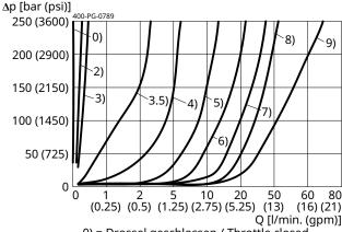
0) = Drossel geschlossen / Throttle closed 1-9) = Drosseleinstellung pro Umdrehung / Throttle setting per revolution
