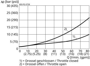
$Q = f(I:\Delta p)$  Flow rate adjustment Adjustment, normal opening Measured with supply channel 1 and 2 = Ø0.28" At constant throttle settings
