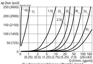
0) = Drossel geschlossen / Throttle closed 1-6) = Drosseleinstellung pro Umdrehung / Throttle setting per revolution
