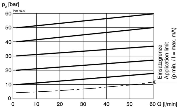
$p = f(Q)$  Druck-Volumenstrom-Kennlinie  $p_N = 63 \text{ bar}$
