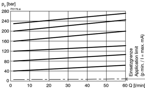
$p = f(Q)$  Druck-Volumenstrom-Kennlinie  $p_N = 300 \text{ bar}$
