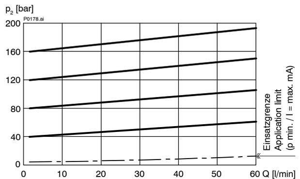
$p = f(Q)$  Druck-Volumenstrom-Kennlinie  $p_N = 230 \text{ bar}$
