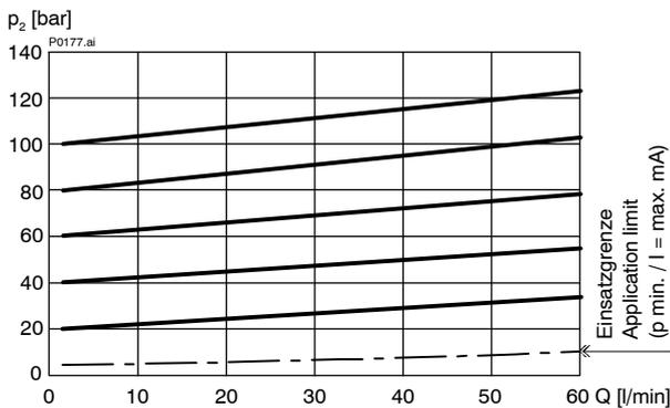
$p = f(Q)$  Druck-Volumenstrom-Kennlinie  $p_N = 160 \text{ bar}$
