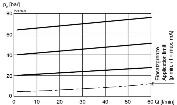
$p = f(Q)$  Druck-Volumenstrom-Kennlinie  $p_N = 100 \text{ bar}$
