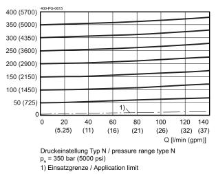
$\Delta p = f(Q)$  Pressure drop-flow rate characteristic  $\Delta p$  [bar (psi)]
