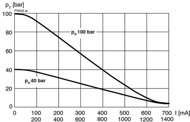
$p = f(I)$  Pressure adjustment characteristic ( $Q = 10$  l/min)
