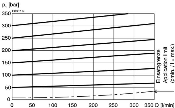
$Q_L = f(p)$  Leakage flow rate characteristic (1 → 2)
