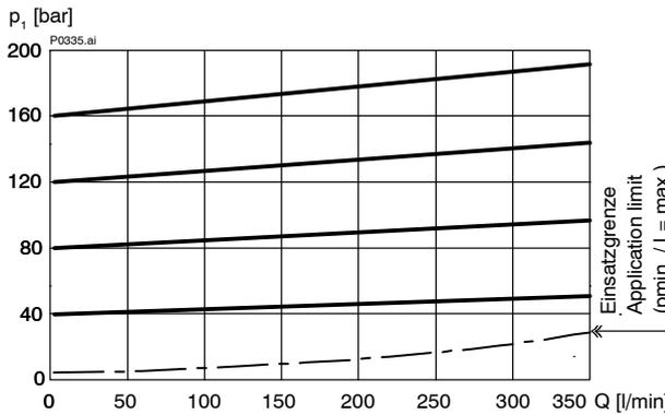
$p = f(Q)$  Pressure - Flow rate characteristic  $p_N = 250$  bar
