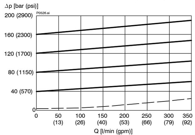
$\Delta p = f(Q)$  Pressure-drop characteristic (100 bar)
