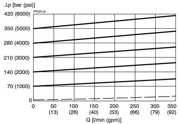
$\Delta p = f(Q)$  Pressure-drop characteristic (250 bar)
