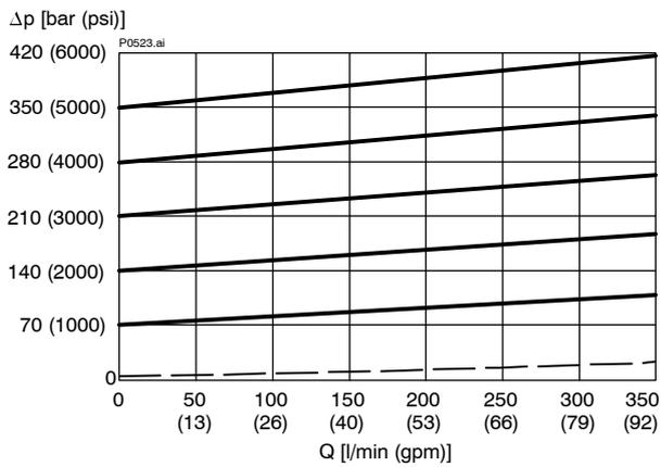
$\Delta p = f(Q)$  Pressure-drop characteristic (350 bar)
