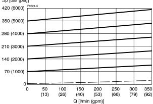
$\Delta p = f(Q)$  Pressure-drop characteristic (160 bar) ∆p [bar (psi)]
