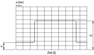
Example – showing the adjustable pressures p1 and p2:
