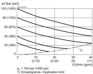
p = f (Q) Pressure-flow rate Pressure range 725...3600 psi
