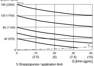
p = f(Q) Pressure - Flow rate characteristic [ $p_N = 100$  bar]  $p_2$  [bar (psi)]
