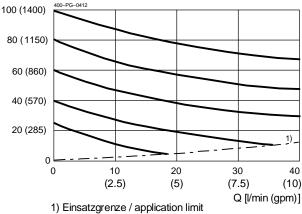
p = f(Q) Pressure - Flow rate characteristic [ $p_N = 250$  bar]  $p_2$ [bar (psi)]
