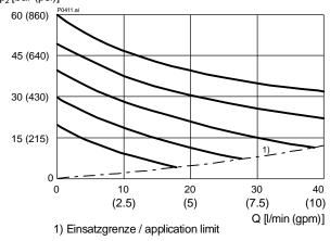
p = f(Q) Pressure - Flow rate characteristic [ $p_N = 160$  bar]  $p_2$  [bar (psi)]
