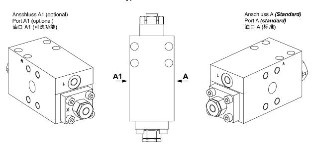
The main port is defined as seen from the perspective of the cover. As standard, the main port A is located on the right side. A variant with main port A1 is available as an option.
