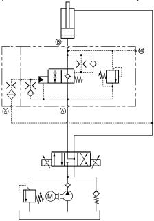
Circuit example for SVZ (B  $\rightarrow$  L), not influenced by return-line pressure, for directional valves with closed-centre spool
