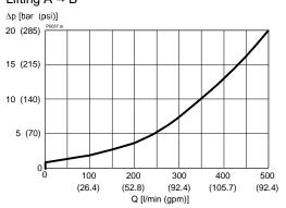
p = f (Q) Pressure - Flow rate characteristic Secondary pressure relief valve SVA / SVT
