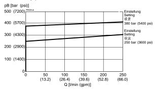
$\Delta p$  = f (Q) Pressure drop - Flow rate characteristic Lowering B  $\rightarrow$  A
