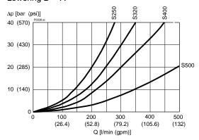
p = f (Q) Pressure - Flow rate characteristic Thermal-expansion pressure relief SVZ
