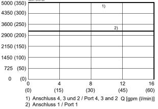
$\Delta p = f(Q)$  Pressure drop-flow rate characteristic
