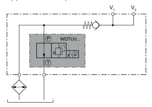
Manifold block with integral cooler-bypass thermostat valve
