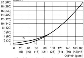
1) 1  $\rightarrow$  2, 2  $\rightarrow$ 1 solenoid energized 2) 1  $\rightarrow$  2 solenoid de-energized
