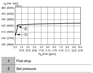
Due to the way the SVX works, a small amount is tapped at port B before the set pressure is reached.
