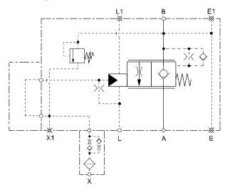
center position and secondary valve connected in series, no pressure summing occurs. There is no need for a largebore, external tank return line.
