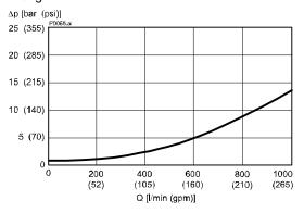
Q = f (pX) Pressure - Flow rate characteristic at 33 bar load pressure
