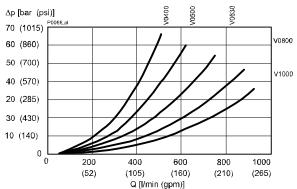
p = f (Q) Pressure - Flow rate characteristic Secondary pressure relief valve SVX
