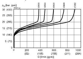
$\Delta p$  = f (Q) Pressure drop - Flow rate characteristic Lowering B  $\rightarrow$  A
