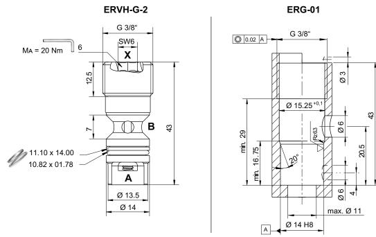
**ERVH-G-2** = check valve / screw-in cartridge valve **ERG-01** = dimension of the cavity for screw-in cartridge valve ERVH-G-2
