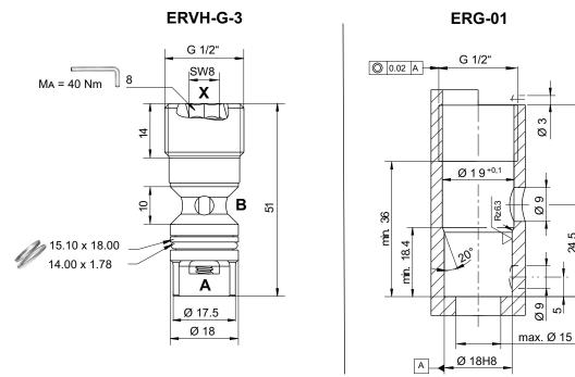
**ERVH-G-3** = check valve / screw-in cartridge valve **ERG-01** = dimension of the cavity for screw-in cartridge valve ERVH-G-3 The dimensions specified apply to the mounted state.
