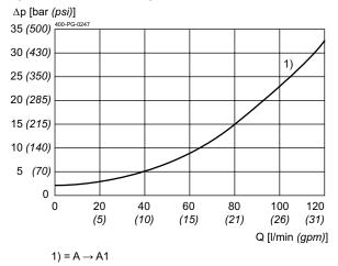
$\Delta p = f(Q)$  Pressure drop-flow rate characteristic  $\Delta p$  [bar (psi)]
