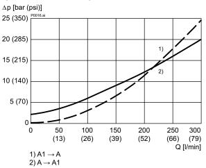
Δp = f (Q) Pressure drop-flow rate characteristic
