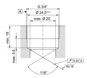
**RKVE-G-16-02-KB** = check valve / screw-in cartridge valve **REG-05-E** = dimension of the cavity for screw-in cartridge RKVE-G-16-02-KB **1** = sealing edge for metal-to-metal sealing
