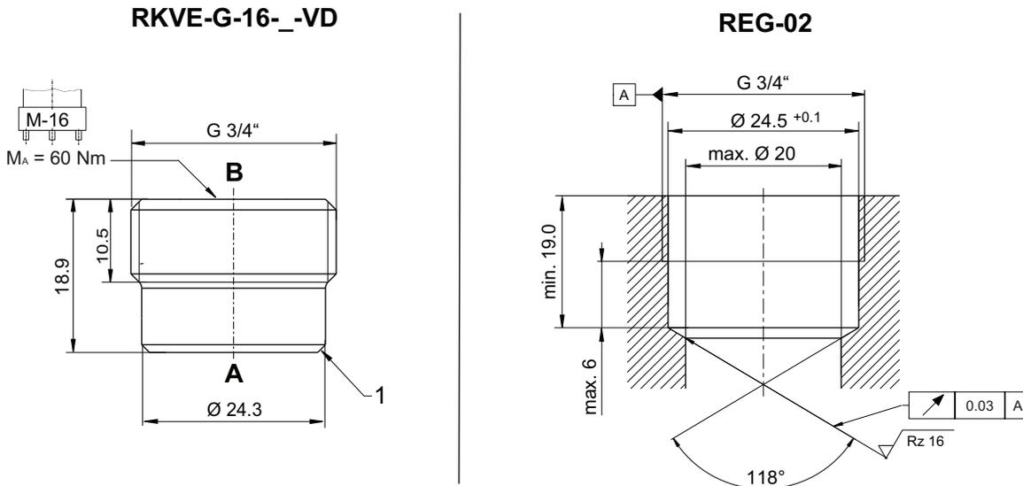
**RKVE-G-16-\_-VD** = check valve / screw-in cartridge valve
