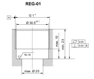
RKVE-G-25-\_\_-VD = check valve / screw-in cartridge valve
