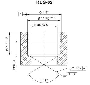
RKVE-G-06-\_-VD22 = check valve / screw-in cartridge valve
