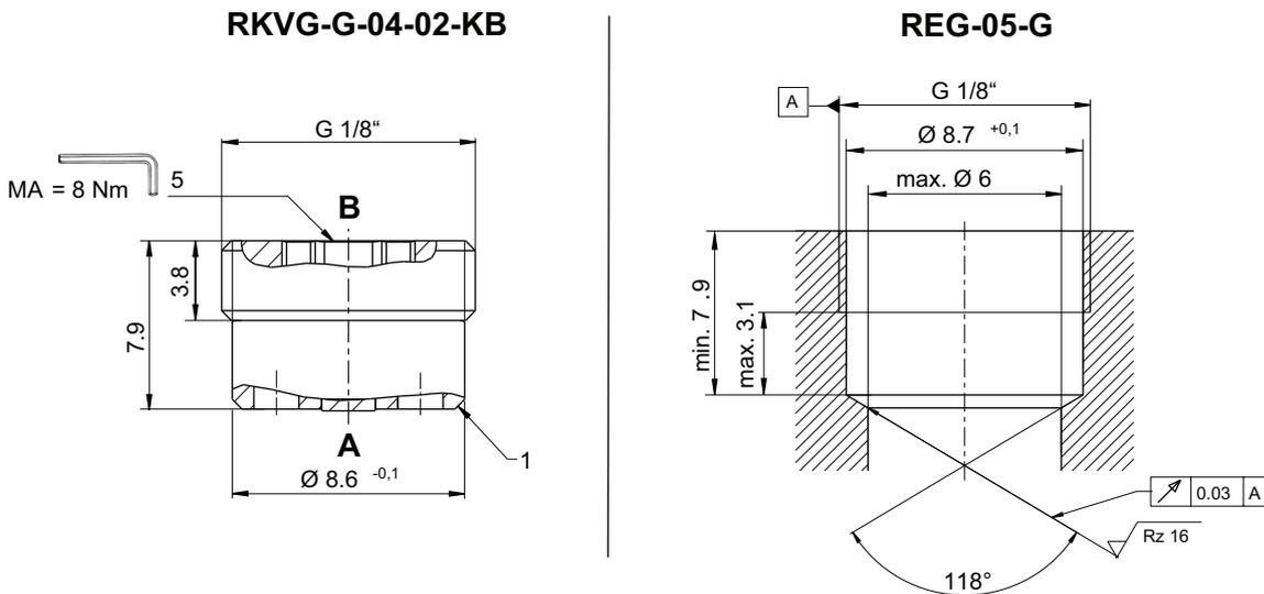
**RKVG-G-04-02-KB** = check valve / screw-in cartridge valve
