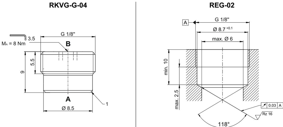
**RKVG-G-04** = check valve / screw-in cartridge valve
