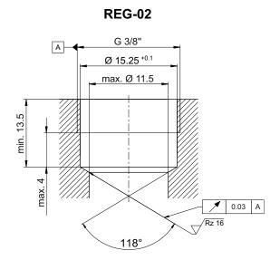
**RKVG-G-08** = check valve / screw-in cartridge valve **REG-02** = dimension of the cavity for screw-in cartridge RKVG-G-04 RKVG-G-08
