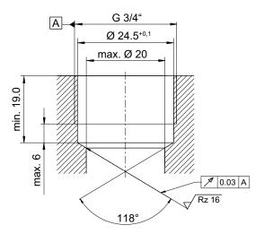
**RKVG-G-16** = check valve / screw-in cartridge valve **REG-02** = dimension of the cavity for screw-in cartridge RKVG-G-16 **1** = sealing edge for metal-to-metal sealing
