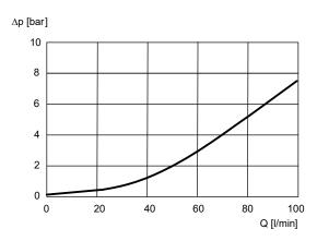
$\Delta p$  = f (Q) Pressure drop-flow rate characteristic Used as preload valve
