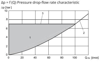
1 = Pressure loss area (The actual pressure-loss characteristic is dependent on the tank pressure at port B)
