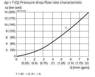
measured with on viscosity 55.0 min 75 (CSt)
