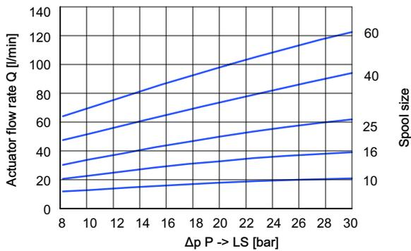
5.1.5.2 Flow characteristic with individual pressure compensator at flange face U
