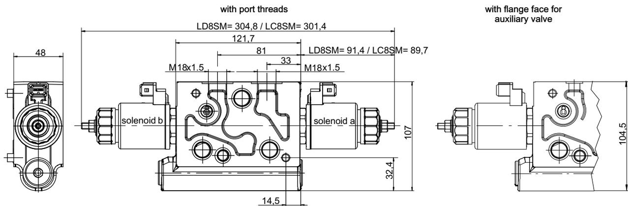
5.2.8.4 LD8S / LC8S-directional valve with integrated pressure compensator and flow cut-off
