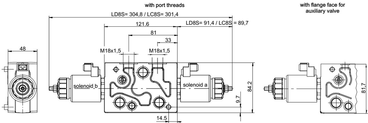
5.2.8.3 LD8SM / LC8SM-directional valve with integrated pressure compensator
