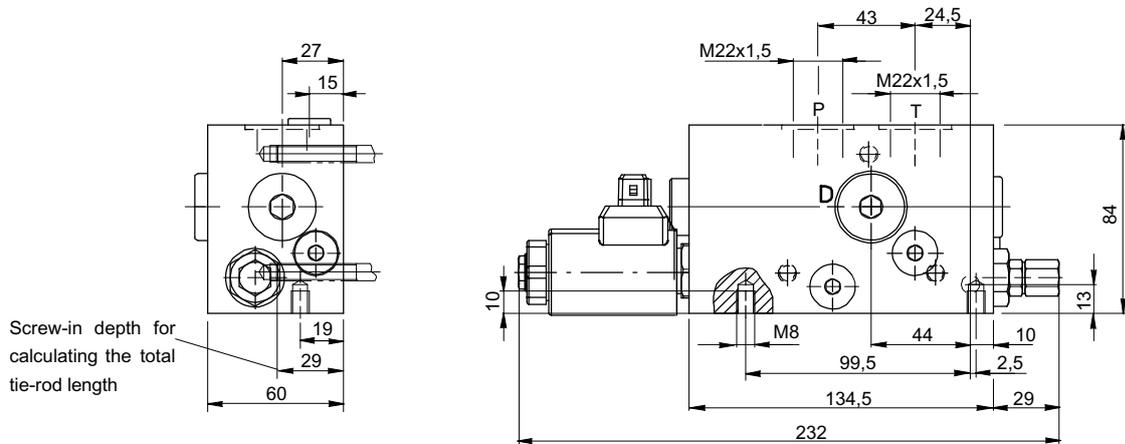
Screw-in depth for calculating the total tie-rod length
