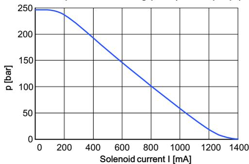
5.2.4.8 Typical pressure profile 3-way pressure control Electroproportional
