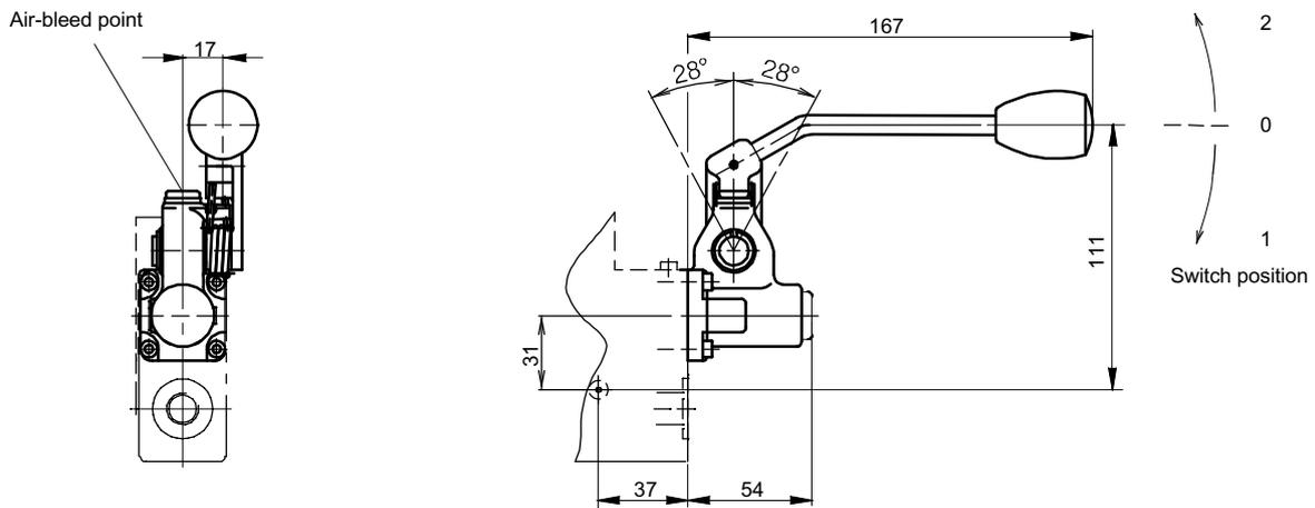
5.4.7.4 Manual override for LH8S-directional valves and spool stroke limiter (LH8S.....-N../16)
