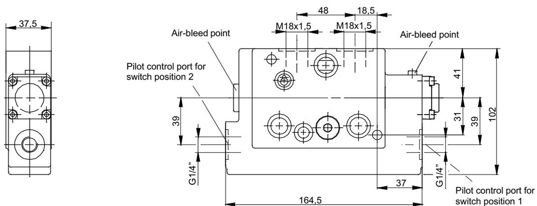
5.4.7.2 LH8S-directional valves (with flange face to bolt-on auxiliary valves)
