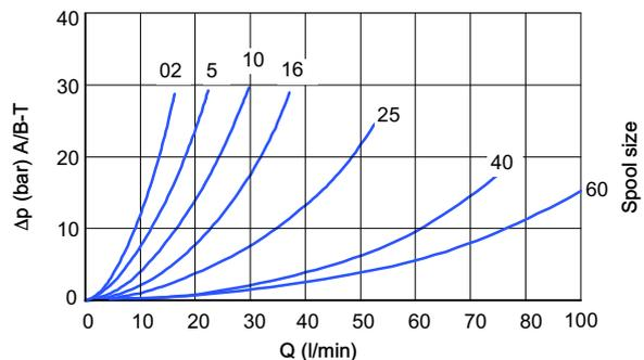
5.2.4.5 Typical flow characteristic curve with flow cut-off function, pressure relief adjustable (manual)
