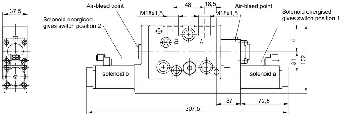
5.3.8.2 LM8S-/ LP8S-directional valve with facility for bolt-on auxiliary valves
