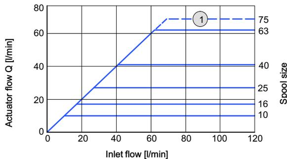
1 Maximum flow rate at directional valve when using the LU8SSKH / SKJ compensator in conjunction with an LU8SSCS inlet section
